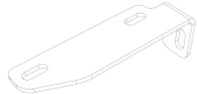
BRACKET, ROPS, ASSEMBLY, RIGHT P/N: 8SV-110-00061-R
