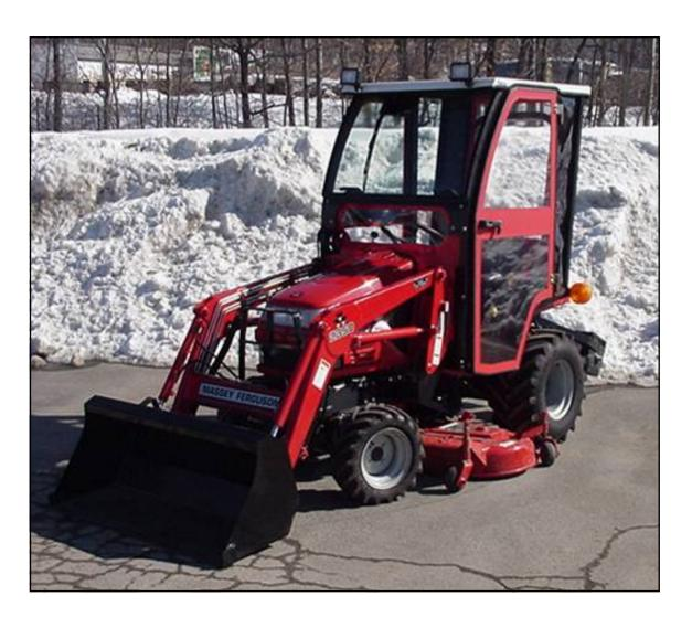
This Curtis Cab is designed and **▲ WARNING** nanufactured for use only as reasonable weather protection. This cab is not applicable, nor should the cab be considered as protection against roll over, collision or other accidents that may result. This cab is NOT a R.O.P.S. cab. Extreme care should be taken when operating and by qualified, experienced operators only.
