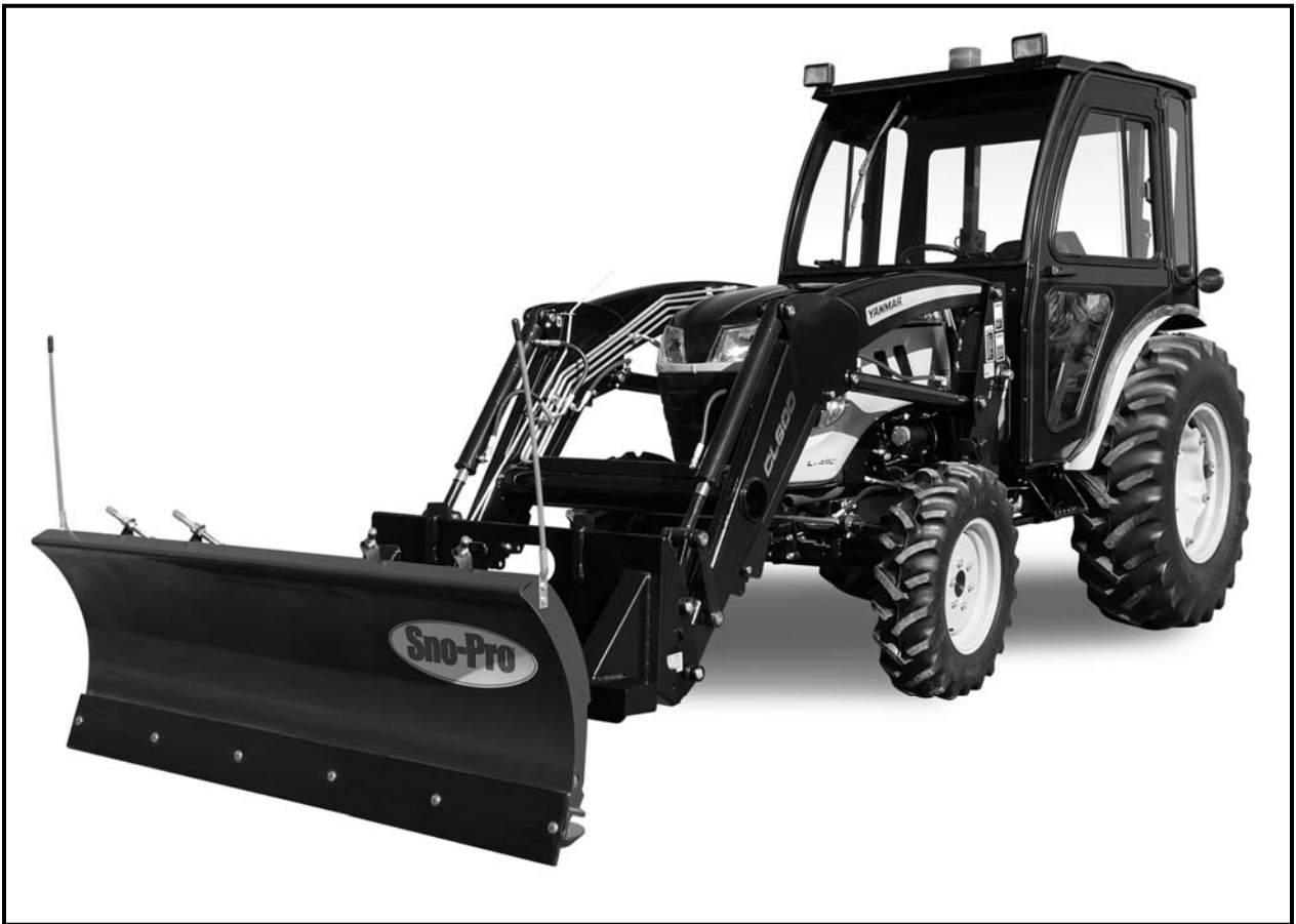
Shown with optional work lights and strobe lights. Additional options available are: heater and rear window wiper (85 degree style). Note: a front windshield wiper (110 degree style) comes standard with this cab kit.
