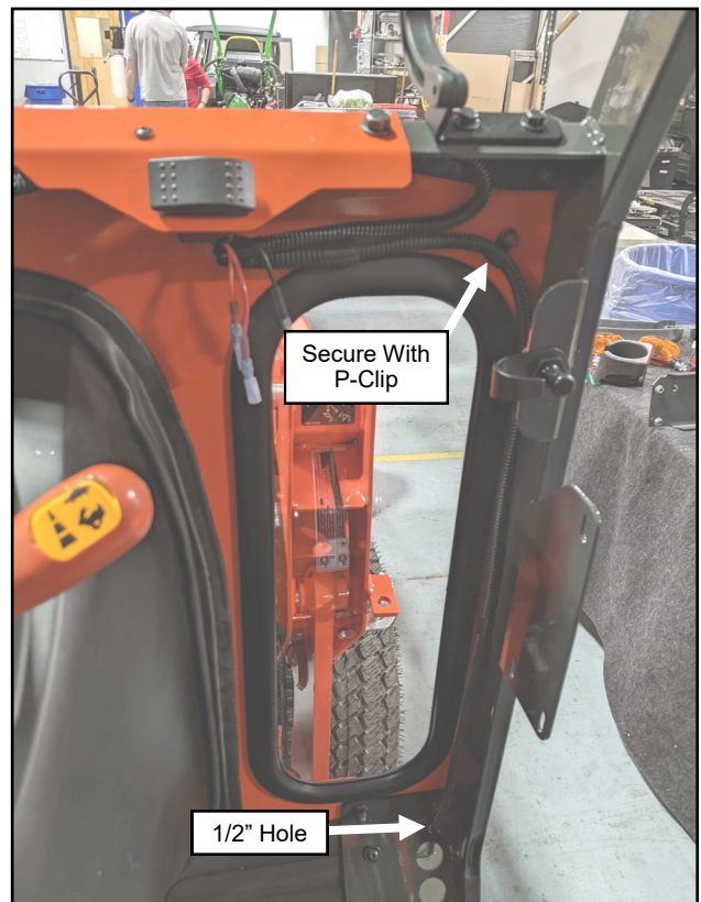
Fig. 13.3 (Harness Runs Down Side Frame)
