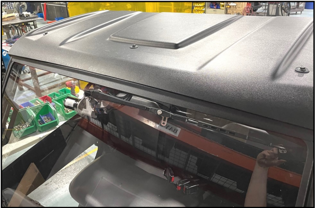
Fig. 2.3 (Install front screws, washers & lock nuts)
