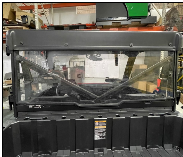
Fig. 2.2 (Install back screws and washers)
