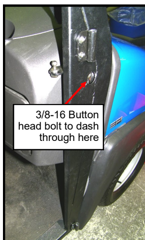
Fig. 2.2: Frame to Dash bolts
