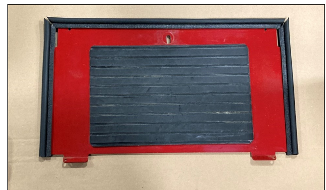
Fig. 2.5 (Install rubber to floor pan)
