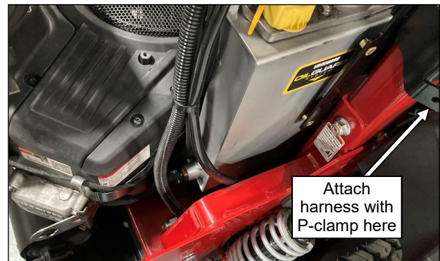
Fig. 6.1 (A/C wire harness)
