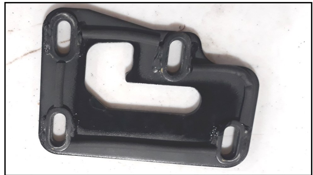
Fig. 2.1 (Guide Plate with Sealing Bulb Adhered)
