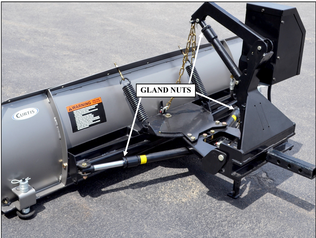
Fig. 11.3 repairing a Hydraulic Cylinder leak
