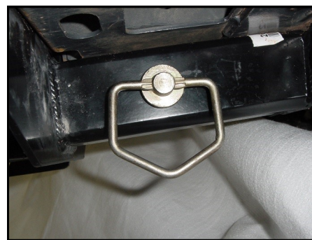
Fig. 2.3—Lift Frame and Receiver Pin (Under Vehicle)
