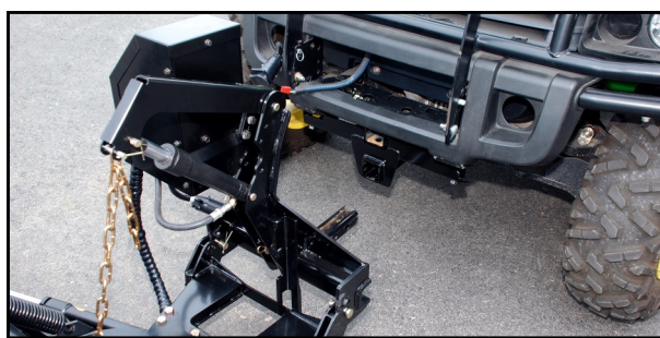
Fig. 2.2—Lift Frame and Receiver Setup
