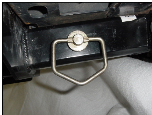
Fig. 1.2—Lift Frame and Receiver Pin (Under Vehicle)
