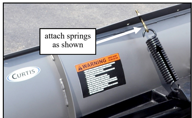
Fig. 2.2—Trip Spring Installation
