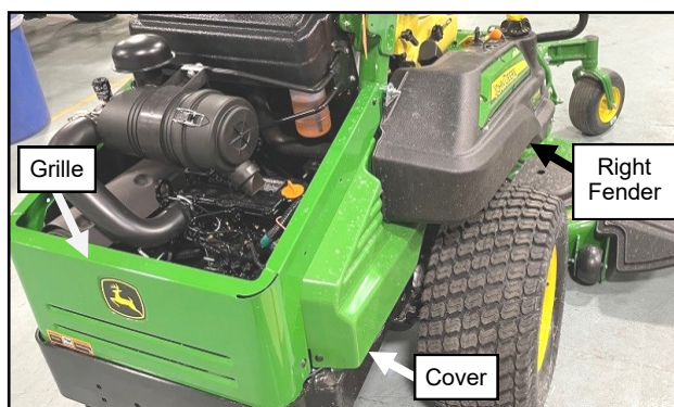
Fig. 1.4 (Remove Cover and Grille)
