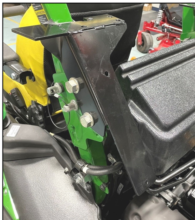
Fig. 1.30a (Install R.O.P.S bracket, left)
