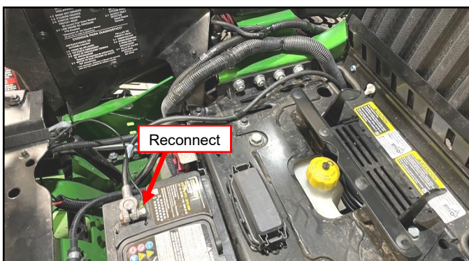
Fig. 2.30b (Run Harness to (-) Terminal on Battery)
