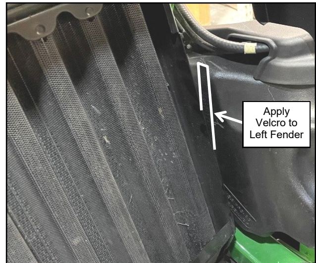
Fig. 2.19 (Install Velcro, Left Fender)
