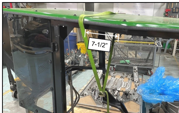
Fig. 2.3 (Position Lifting Strap)
