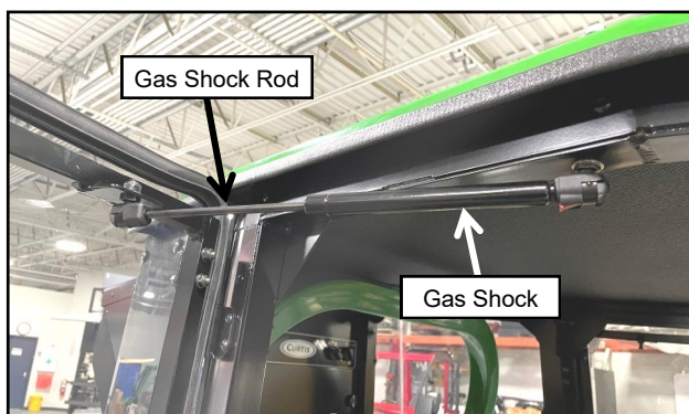
Fig. 2.36b (Install Door Gas Shock, Right)
