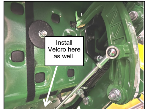
Fig. 2.39a (Under floor Velcro position)
