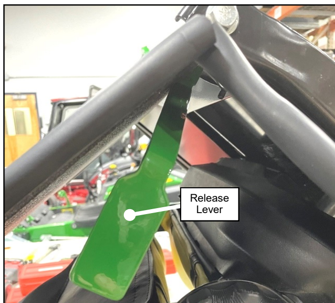
Fig. 1.28 (Install Release Lever)
