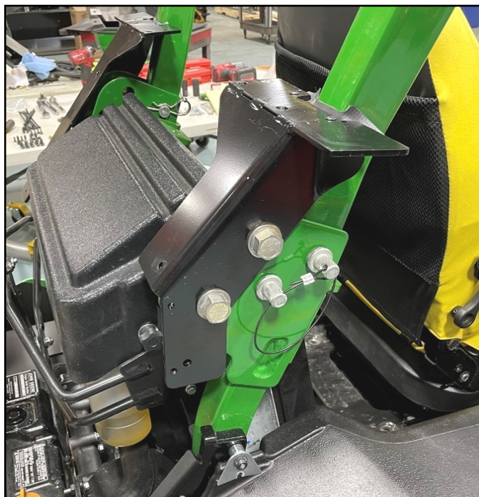
Fig. 1.30b (Install R.O.P.S bracket, right)
