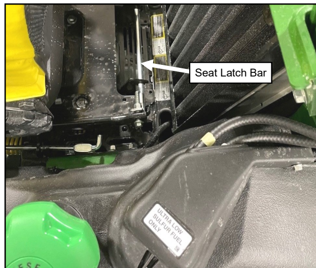
Fig. 1.18 (Tilt Seat Forward)
