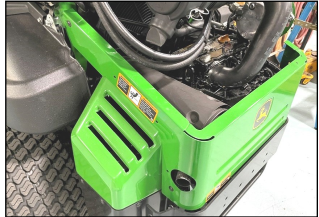
Fig. 2.31 (Install Re-Worked Grille)
