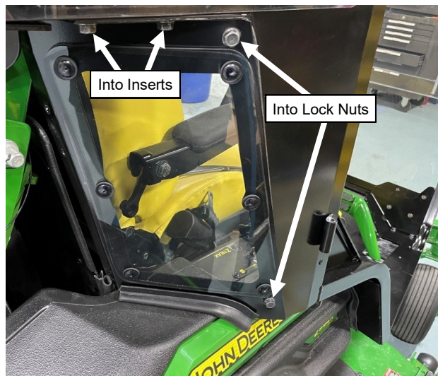
Fig. 2.15 (Install Right Filler)
