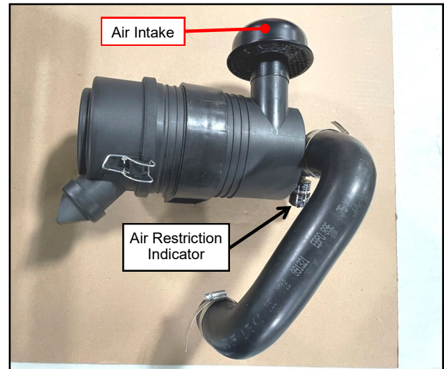
Fig. 2.23b (Reconfigure Air Cleaner, New)
