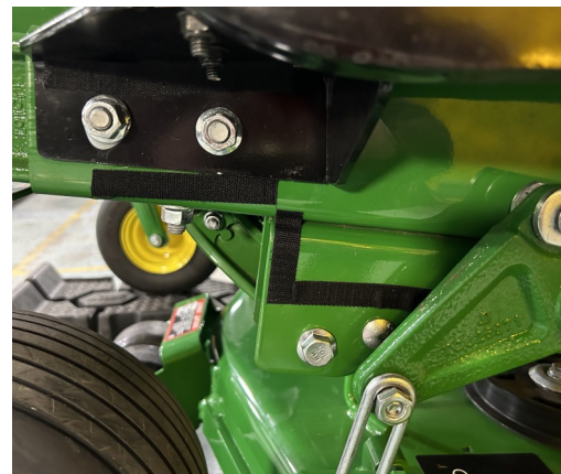
Fig. 2.39b (Velcro on left frame)
