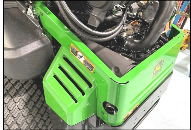
Fig. 2.31 (Install Re-Worked Grille)
