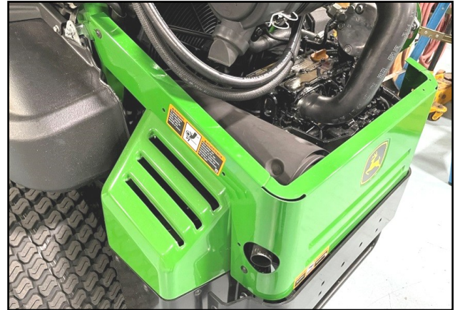
Fig. 2.31 (Install Re-Worked Grille)
