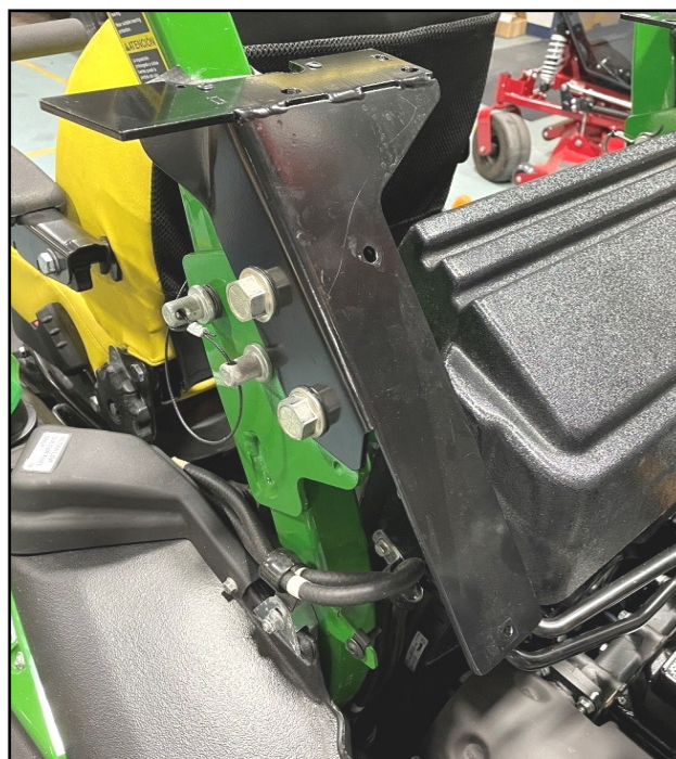
Fig. 1.30a (Install R.O.P.S bracket, left)
