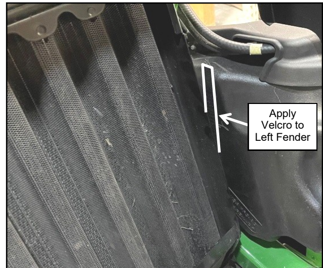
Fig. 2.19 (Install Velcro, Left Fender)
