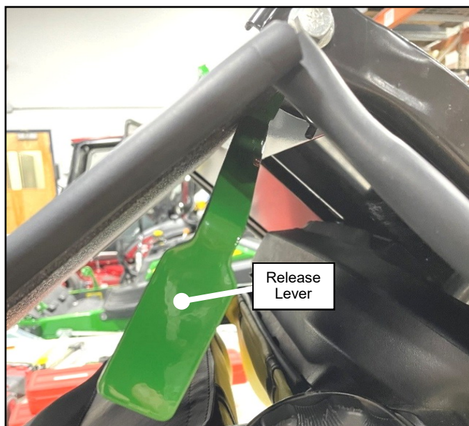
Fig. 1.28 (Install Release Lever)
