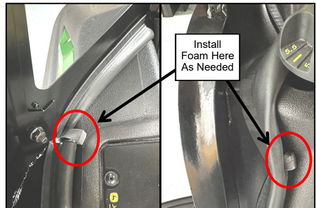
Fig. 2.35b (Install Foam on Right Fender)
