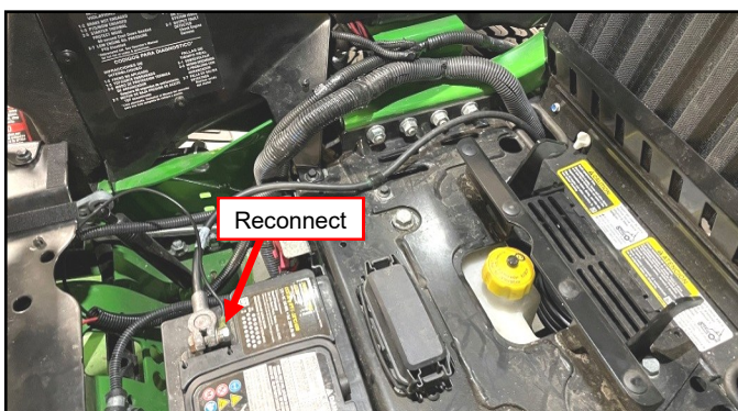
Fig. 2.30b (Run Harness to (-) Terminal on Battery)
