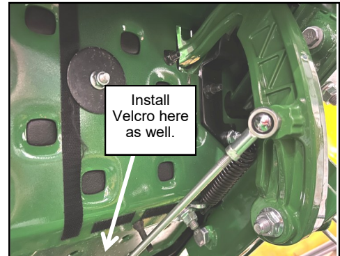
Fig. 2.39a (Under floor Velcro position)
