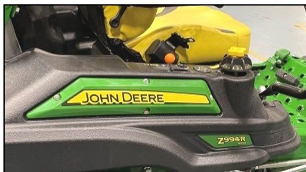
Fig. 1.12 (Re-Install Right Fender)
