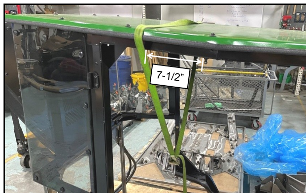
Fig. 2.3 (Position Lifting Strap)
