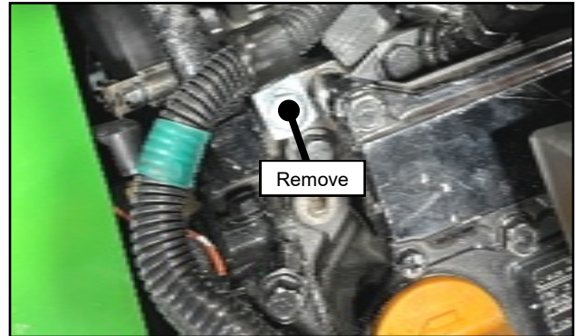
Fig. 1.3 (Remove Screw and P-Clamp)
