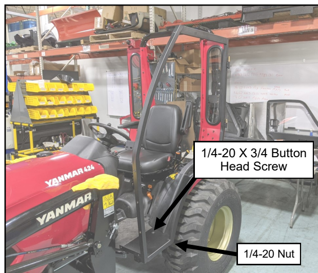
Fig. 4.2 (Install Left Side Frame)
