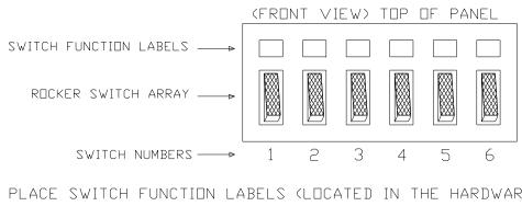
PLACE SWITCH FUNCTION LABELS (LOCATED IN THE HARDWARE BAG) IN THE CORRECT LOCATIONS ACCORDING TO THE SWITCH NUMBERS.
