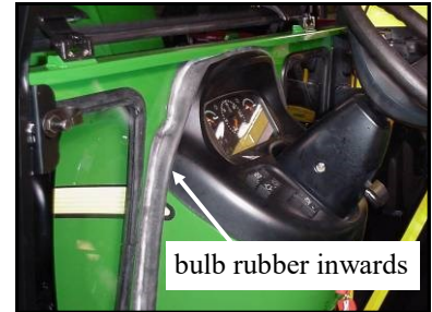
Fig. 3.4 front cowl installed (20 series shown)
