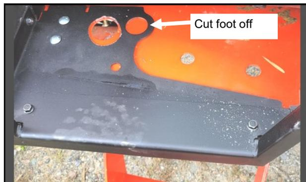
Fig. 2.1 (Modify floorboard mounts)
