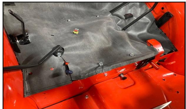
Fig. 16.5 (Install Under Seat Filler)
