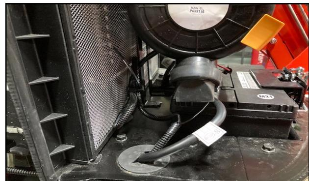
Fig. 13.9 (Coil Wires Behind Battery)
