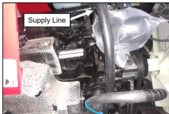
Figure 18.12a (Supply Line Routing)
