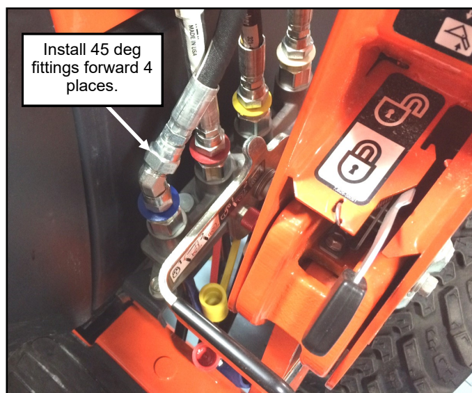
Fig. 1.12b (lever quick coupler, w/ 45 deg fitting - right)
