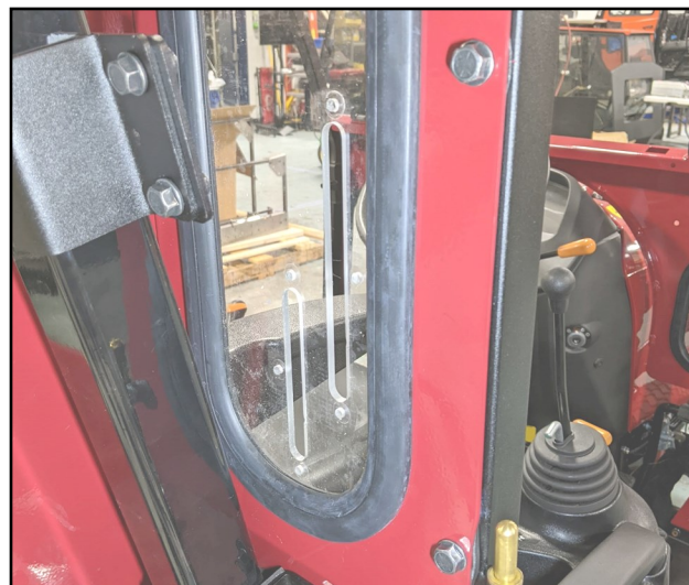
Fig. 3.1 (Remove trim ring and rubber seal)
