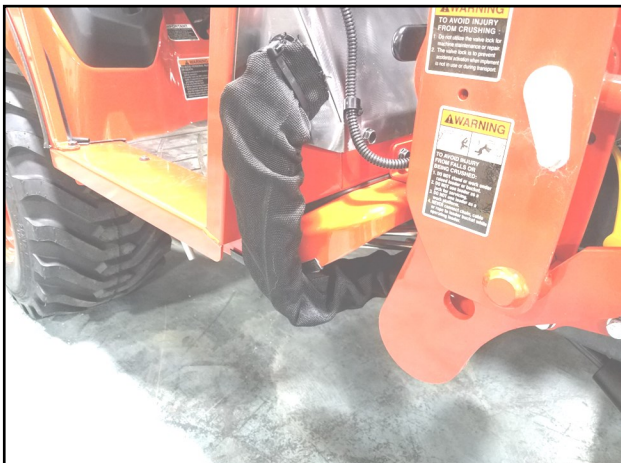
Figure 20.11 (Cover Hoses and Fittings with Mesh)
