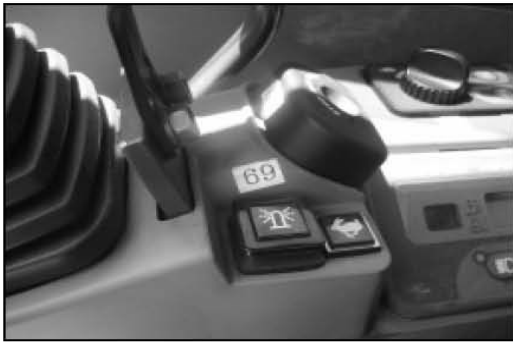
Fig.10. To ensure proper installation before tucking away wires. Connect the (-) battery terminal, Turn the ignition to the accessory or start position. Depress the strobe light button; the Strobe Light will light up.
