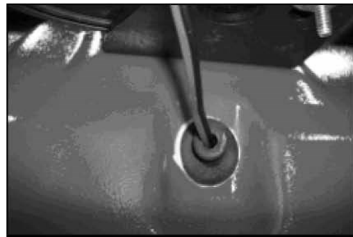
Fig.11. Wind in the left over wires from strobe light into the cab. Plug in the rubber plug, make sure that it seals properly.
