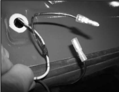
Fig.4. Remove rubber plug from cab, and pull out the wire harness all the way out revealing the BLUE and BLACK wires.
