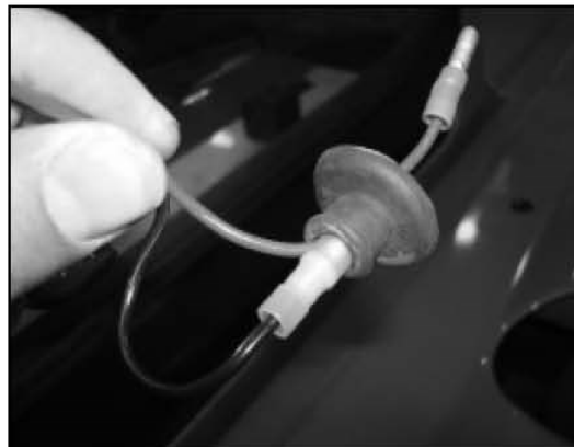
Fig.7. Insert black and blue wires from strobe light through the rubber plug. (This step could be conducted before step 5)
