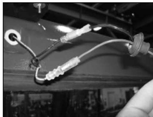
Fig.9. Plug in bullet connectors, male to female.
