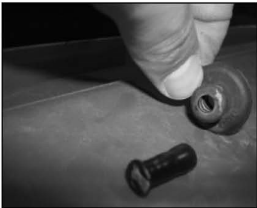
Fig.6. Remove insert from rubber plug.
