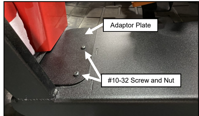
Fig. 18.1 (Install Adaptor Plate, Right)
